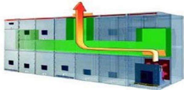
Figure 4 – Illustration of Arc Resistant Venting
