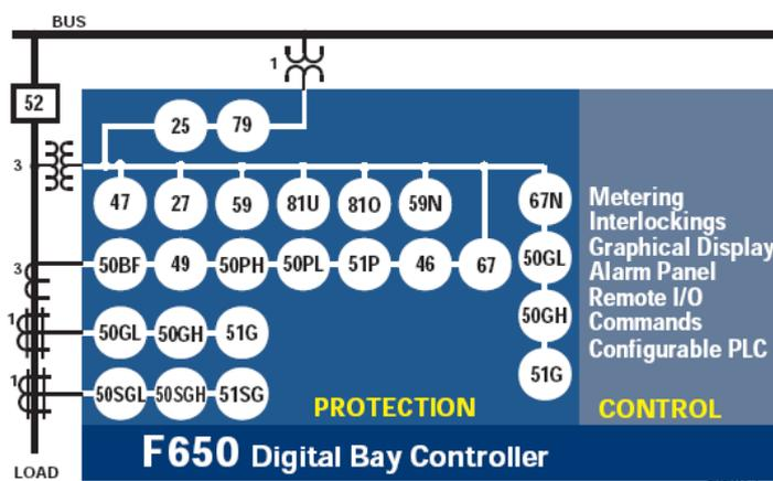
Fig. 3 F650 Function Block Diagram
