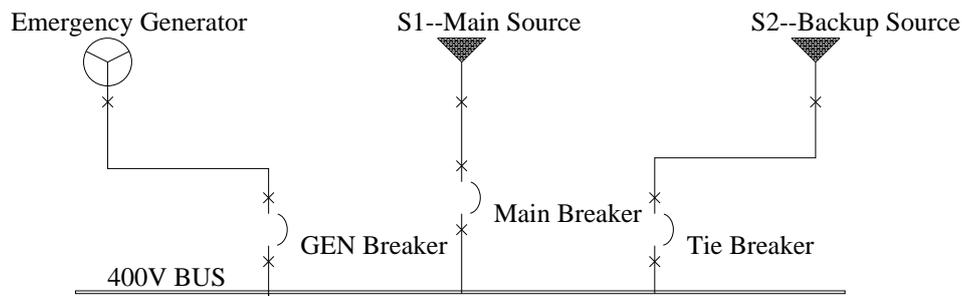
Fig. 1 Simplified Typical IBC LV Switchgear 1-Line
