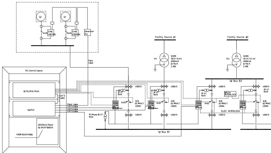
Fig. 2 Simplified 1-Line For Parallel-Capable IBC System
