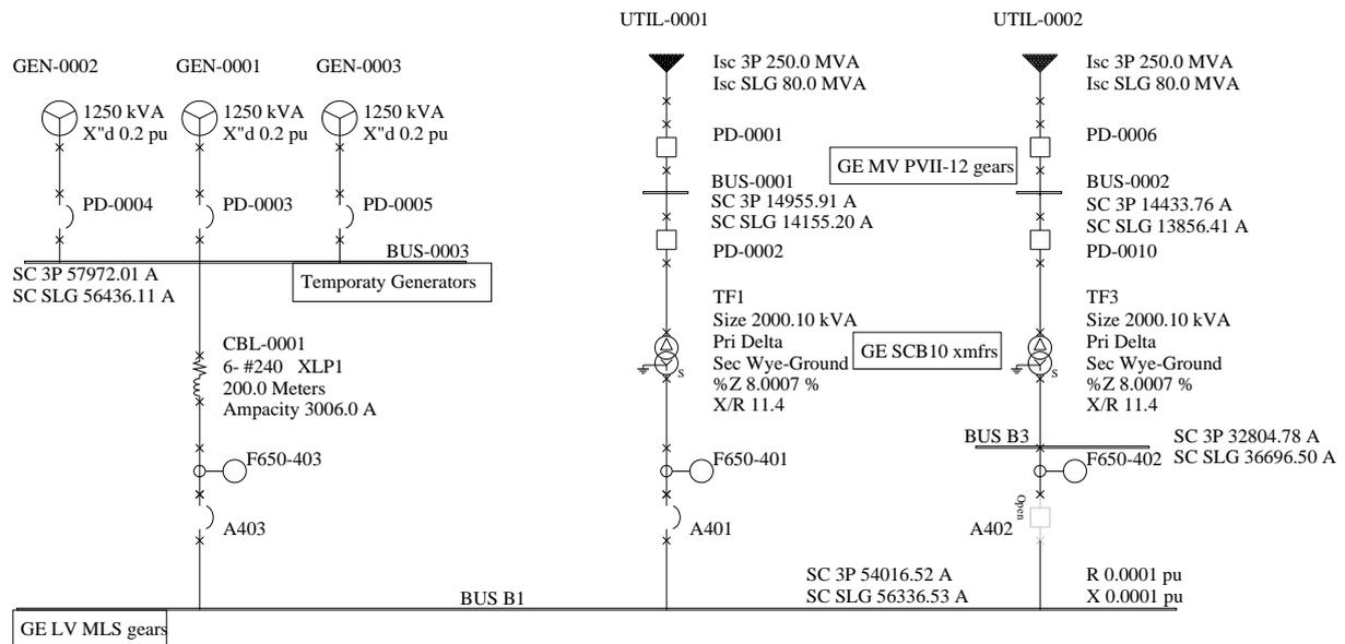
Fig. 4 Short-circuit Model 1-Line
