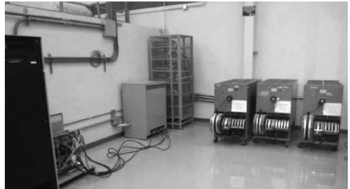
Non-Linear Test Lab Showing Harmonic Generators
