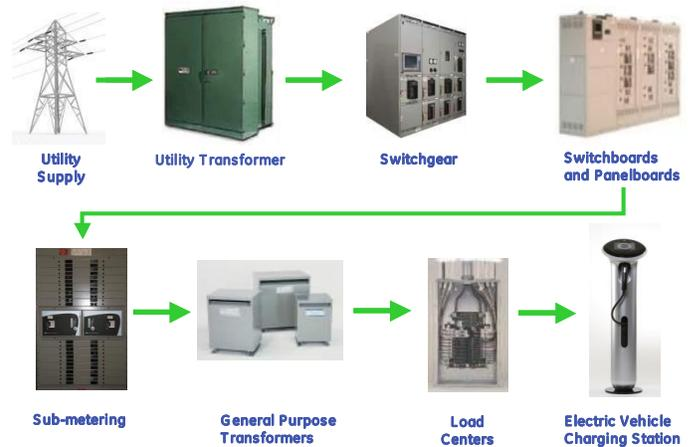
Figure 5 – Typical EVSE Equipment
