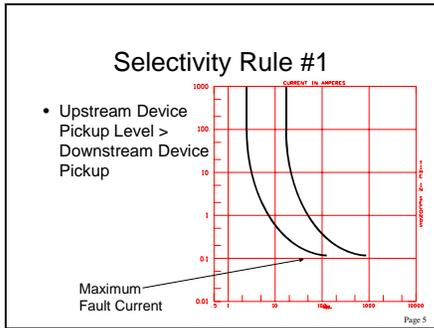
Fig. 2 – Creating selectivity by proper selection of pickup settings.
