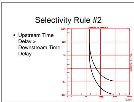
Fig. 3 – Creating selectivity by proper selection of delay settings.
