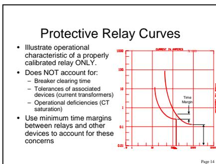
Fig 7. Protective Relay Time Margins
