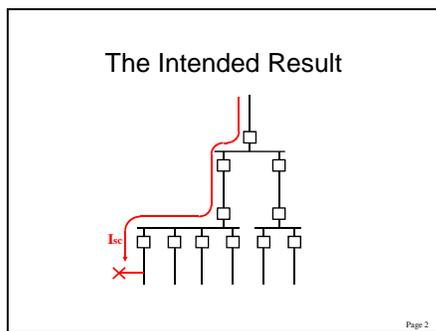
Fig. 1 An example of short circuit flow in a radial system
