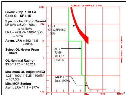
Fig. 9 – A motor load and its protection
