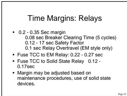
Fig. 8 – Recommended relay time margins
