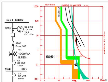
Figure 11 – Unit substation settings
