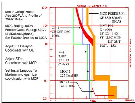
Fig. 10 – Adding the feeder breaker supplying the motor control center
