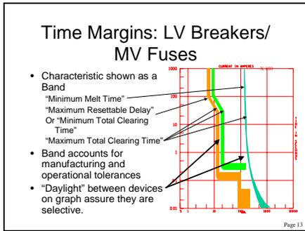
Fig. 6 – Overcurrent device curves with minimum and maximum clearing times
