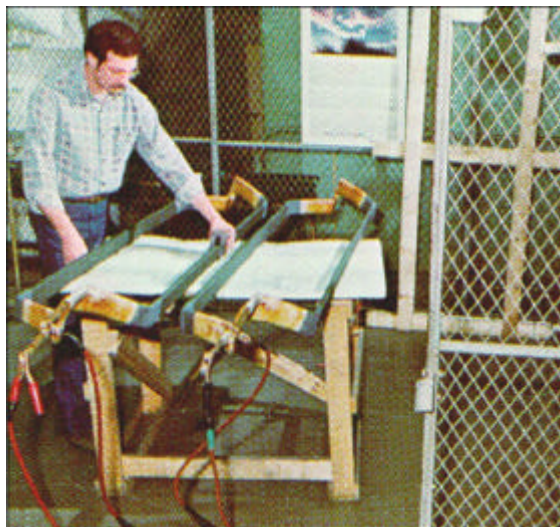
Coils are tested at voltages well above IEEE standards.
