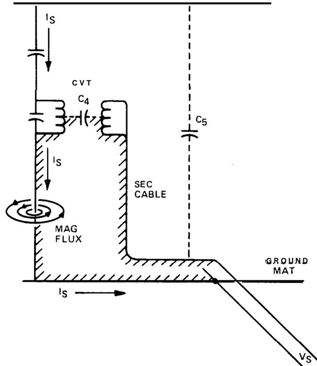
Figure 7. Transient Coupling to the CVT Secondary Circuit
