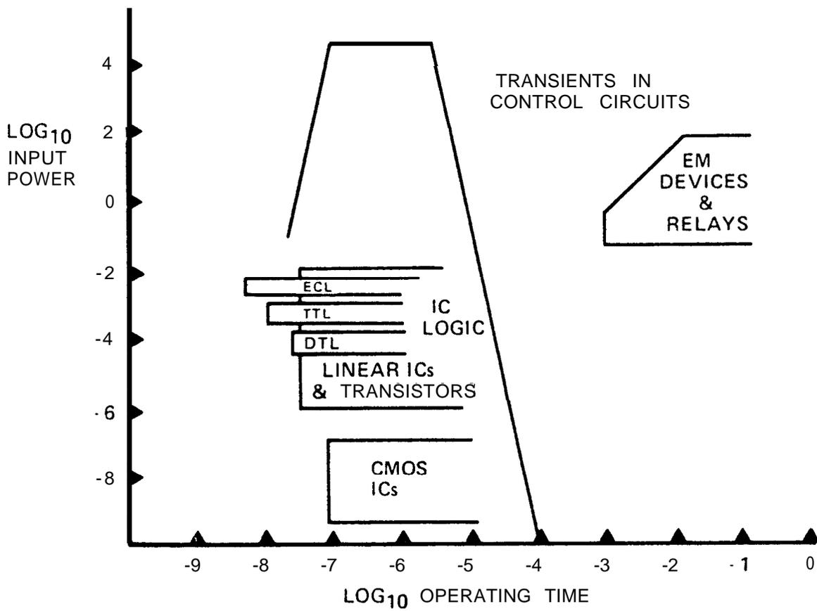
Figure 1. Comparative Response -- Electromechanical and Static Devices
