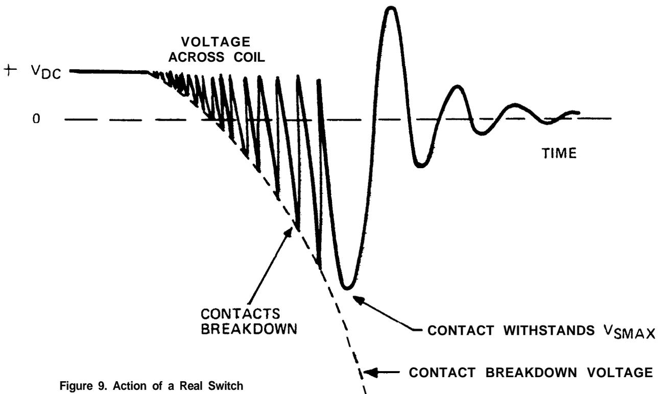
Figure 9. Action of a Real Switch
