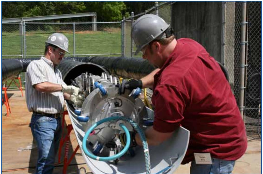
Figure 2. 24-inch Robot Tool w/Slofec insp. tech. tested at EPRI for Buried Pipe Inspection. Photo courtesy of GE
