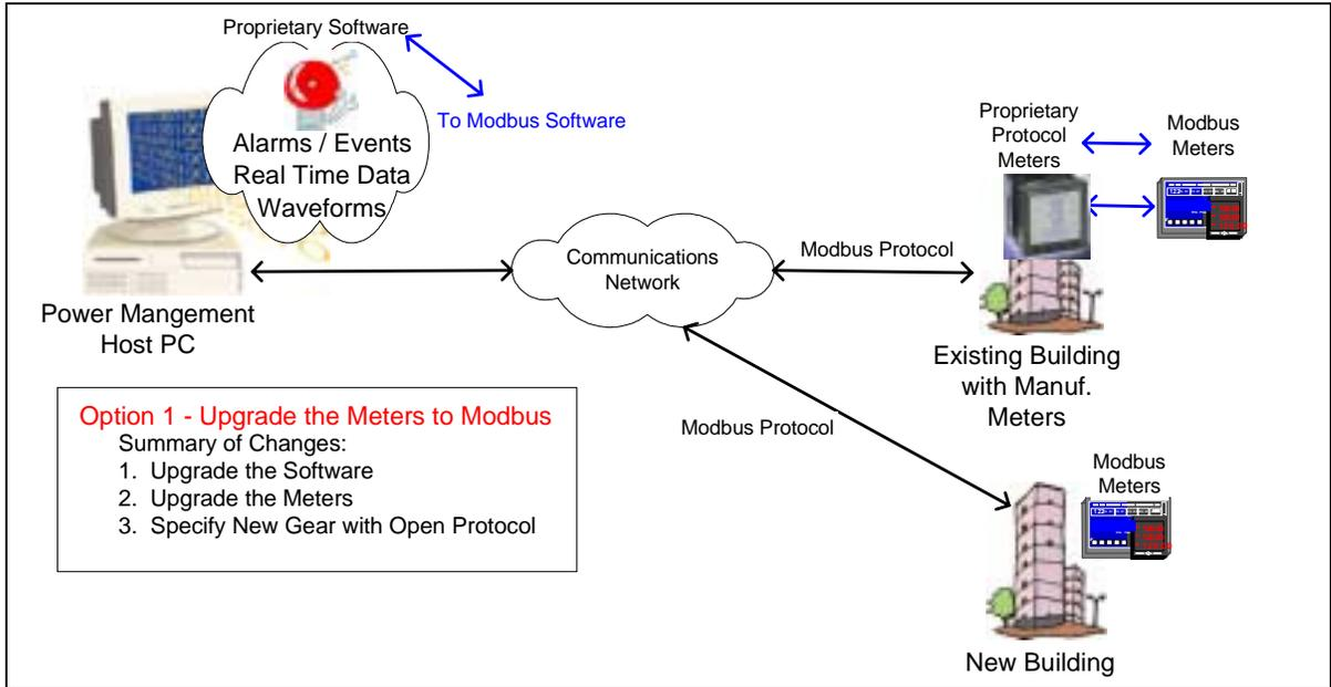
Figure 3 – Option #1 Upgrade the Meters to Modbus
