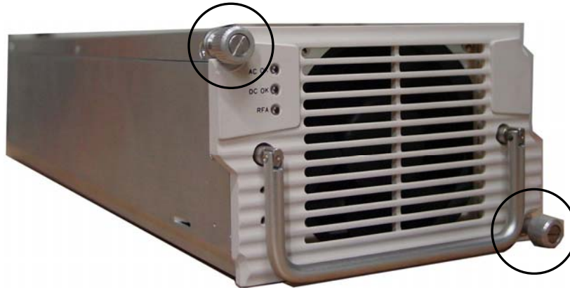
Figure 2-15: Retaining screw locations on the rectifier module
