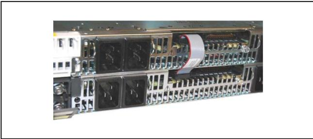
Figure 15 - Shelf-to-shelf ribbon cable of connector J2
