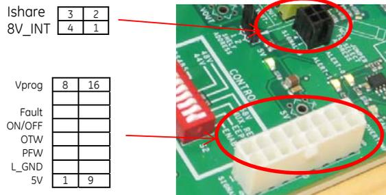
Figure 8 – Signal connector
