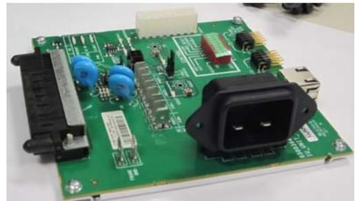
**Figure 2 – Single Module CPL Interface card for rectifiers**
