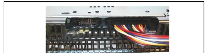
Figure 14 - Control cable plugged into the J1 connector
