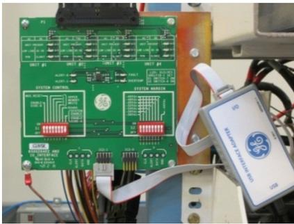
Figure 12 - CPL Shelf module connected to the GE Adapter
