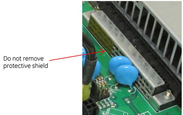
Figure 5 – Protective Shield
