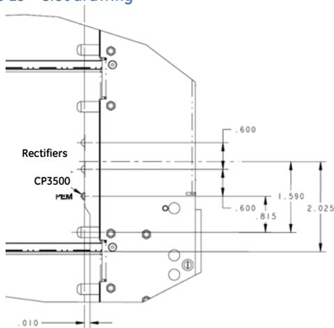
Figure 20 - Module type selector mechanical Key
