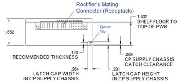
Figure 21 - View looking from the front without a module
