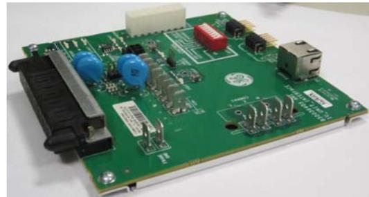
**Figure 3 – Single Module CPL interface card for DC-DC converters**
