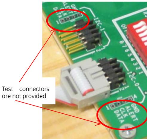
Figure 7 – Signal Connections
