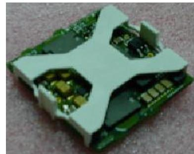
Fig. 9. Example of pick-and place fixture in TEPS power modules
