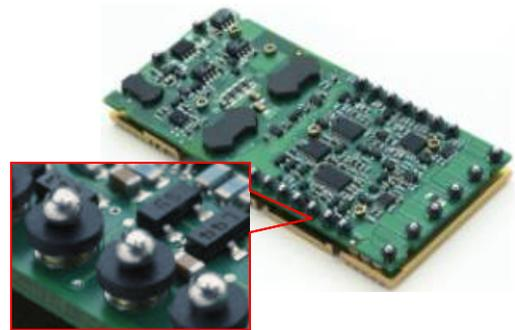
Fig. 1. Picture of a sample module with CPSB
