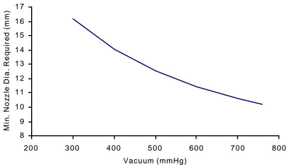
Fig. 10. Nozzle diameter vs. vacuum
