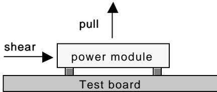
Fig. 6. Sketch of pull and shear test setup
