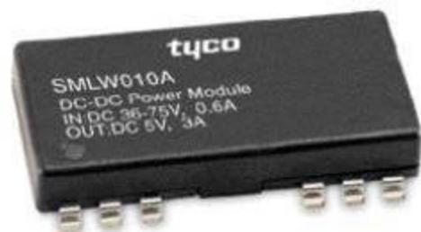
Fig. 2. Picture of SMLW010 power module
