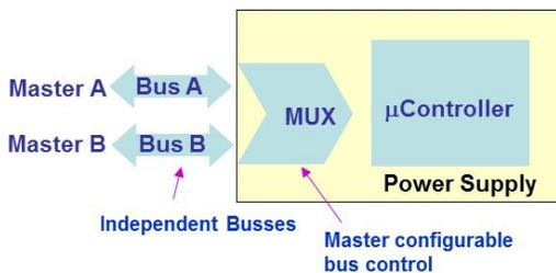
Diagram showing the dual I<sup>2</sup>C bus system.
