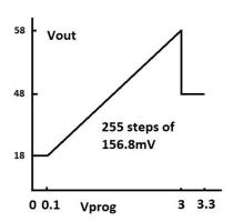
An open circuit on this pin reverts the voltage level back to the original setting of 48V
