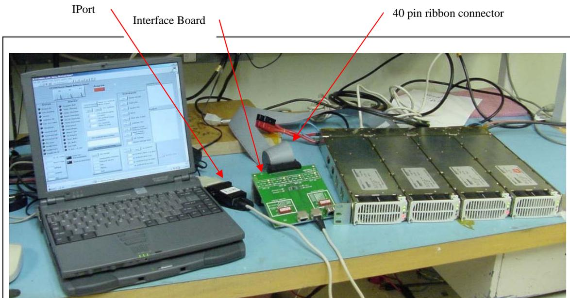
Figure 2: A complete communications system set-up
