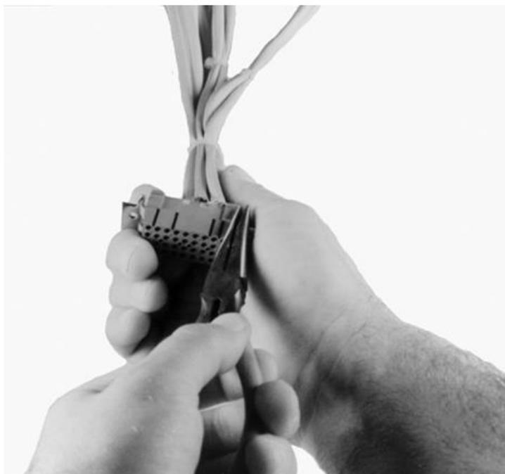
*Fig. 1c. Adapter Bracket Locking Tabs*
