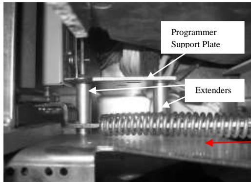
Figure 16: Top view of mounting plate and support bracket (RL-3200 & RL-4000)
