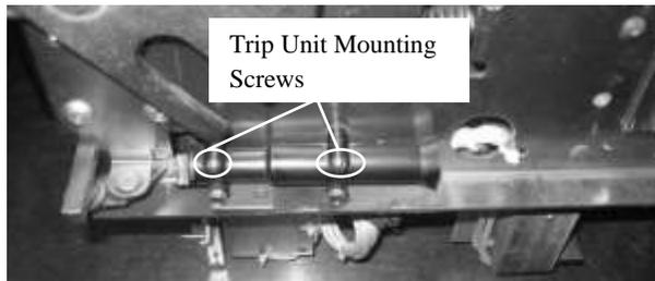
Figure 18: Side of breaker showing black tube like piece (RL-3200/4000 only)
