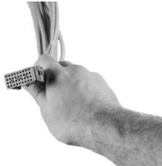
Figure 7. 36-pin trip unit connector
