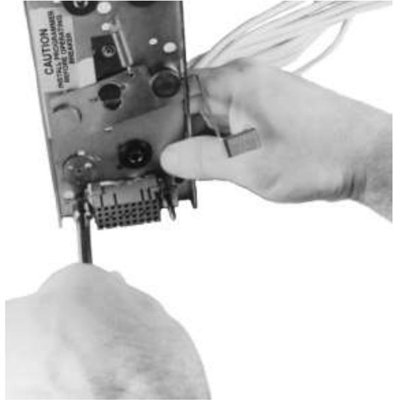
*Figure 10. Installing the push nuts onto the guide pins*
