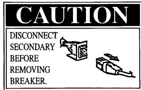
Figure 25. Caution label to be applied to the breaker and compartment door
