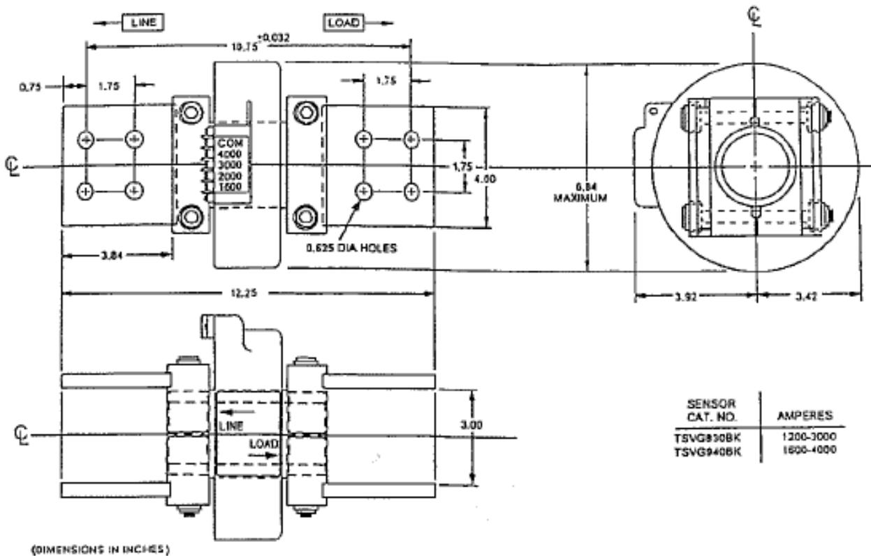
Figure 21. Neutral sensor outline for 3000A through 4000A breakers
