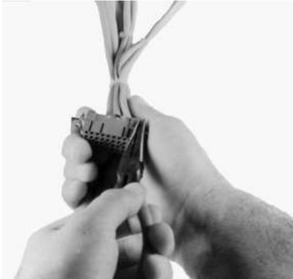
*Figure 11. Adapter bracket locking tabs*
