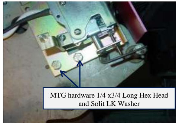
Figure 6: Flux Shifter mounting
