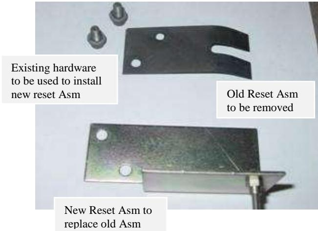
Figure 3: Old and New Reset Assembly
