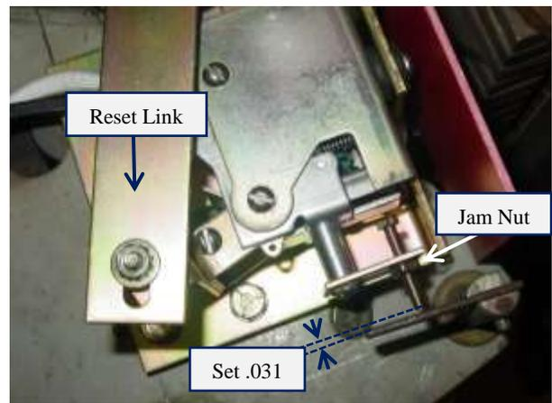
Figure 8: Installing Reset Link
