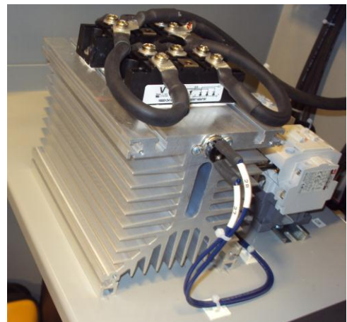
Figure 6.5 - External Rectifiers and PreCharge Assembly
