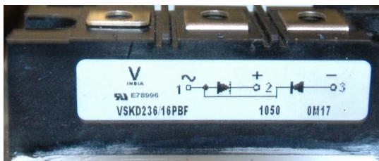
Figure 6.6 - External Rectifier sample
