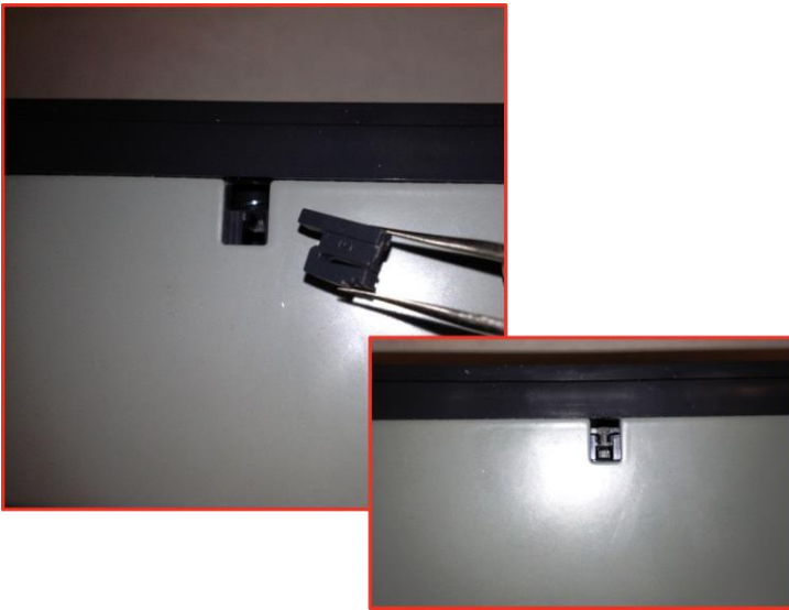
Figure E: Re-insertion of Locking Pin
