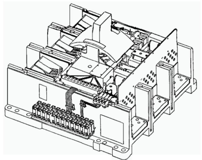
Fig. 2 Ground Fault Breaker with Cover Removed
