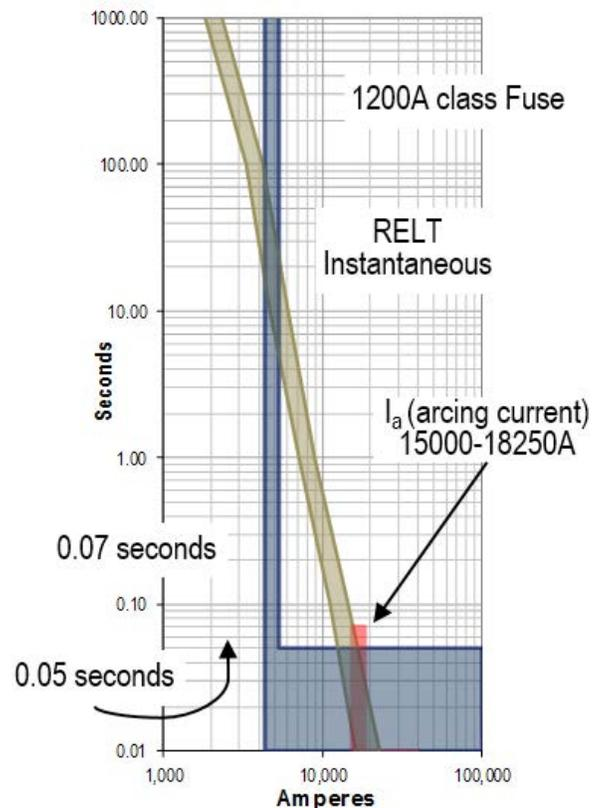
Figure - 1: 1200A class L fuse shown with GE HPC RELT instantaneous set at 4800A with 15kA-18kA arcing current.
