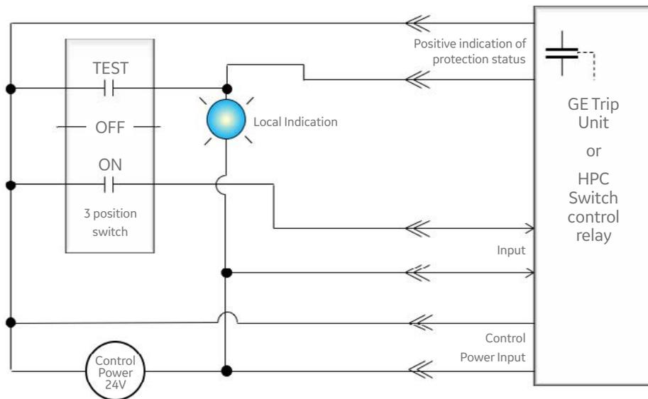
Figure - 4: RELT control circuit showing switch and blue indicating light.
