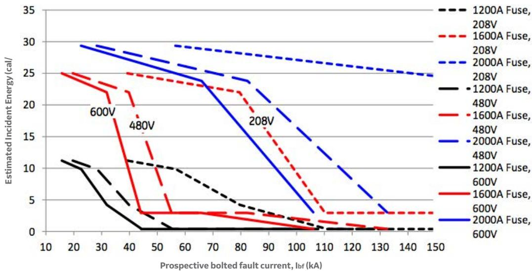
Figure - 2: Plot of IEEE 1584 fuse equations at 600V. Transposed for 480V and 208V arcing current.
