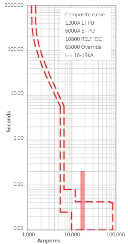
Figure - 5: Circuit breaker without RELT function and arcing current at ~16kA-19kA.
