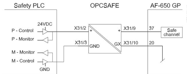
Wire inserting in OPCSAFE
