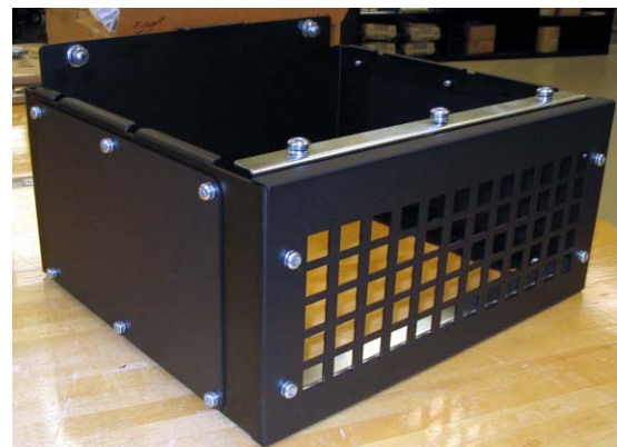
Photo 3. Completely assembled pedestal
