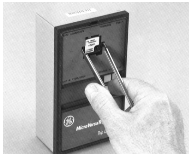
Figure 2. Rating Plug removal.
