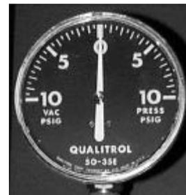
Figure 3. Pressure vacuum gage accessory.
