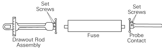
Figure 10. Loadbreak dry-well fuse replacement.
