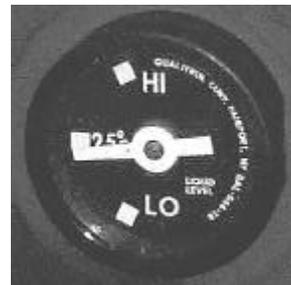
Figure 2. Liquid-level gage accessory.
